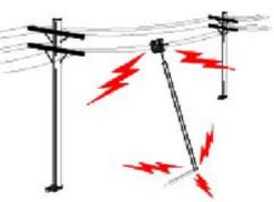
The horizontal distance from a tower, mast or antenna to the nearest power line should be at least twice the total length of the mast/antenna combination. This will ensure that the mast will not contact power if it falls either during installation or later.
