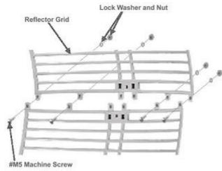
Assemble the halves of the Reflector Grid using (4) #M5 machine screws with lock washers, flat washers and nuts as shown.
