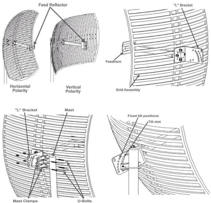
Install the (2) Mast Clamps on the U-Bolts as shown and fasten to the "L" Bracket using (4) lock washers and (4) Nuts.
