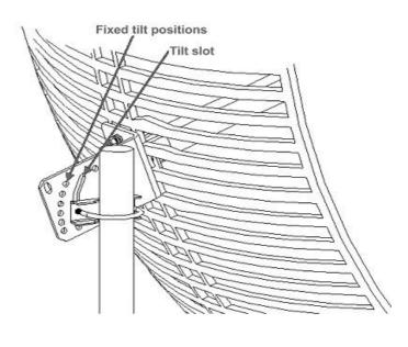
Install the (2) Mast Clamps on the U-Bolts as shown and fasten to the "L" Bracket using (4) lock washers and (4) Nuts.
