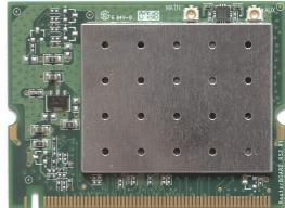
This mini PCI adapter, RouterBOARD R52 contains a dual-mode single chip MAC/BB/Radio for IEEE 802.11a, 11g and 11b Wireless LAN. It can support high-speed data transmission of up to 54 Mbps in the 2.4GHz and 5GHz frequency bands based on 802.11b/g and 802.11a respectively.
